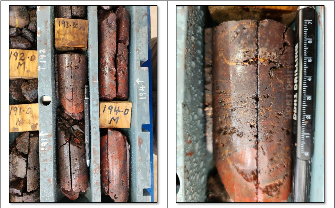
IMAGE 4 a and b: Hematite, quartz, jasper, copper sulphide, copper breccia (BBDD0050 @194m).
