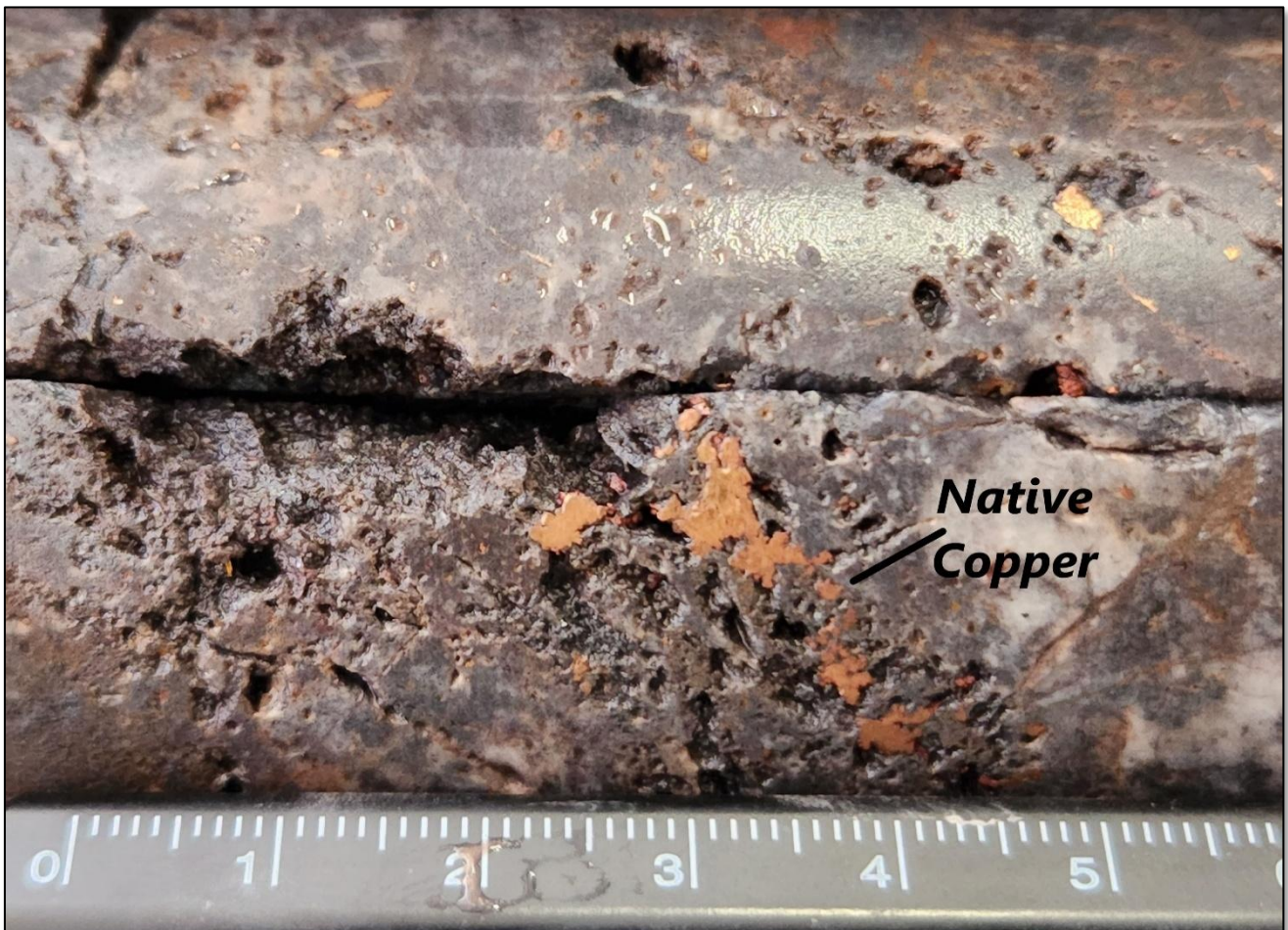
IMAGE 2: BBDD0050:193.3m Native copper and copper-sulphides in quartz-hematite-jasperoid breccia
