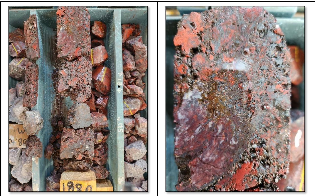
IMAGE 3 a and b: Hematite, quartz, jasper, copper sulphide, copper breccia (BBDD0050 @188m).
