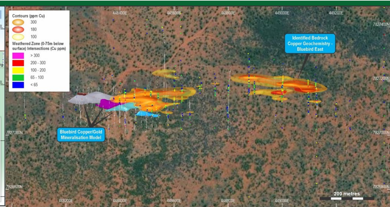
Plan View showing bedrock copper anomalism models (200 and 300ppm) from previous drilling 0-50m below surface data only. 3-D modelled Bluebird high grade mineralised zones shown in blue-purple-grey
