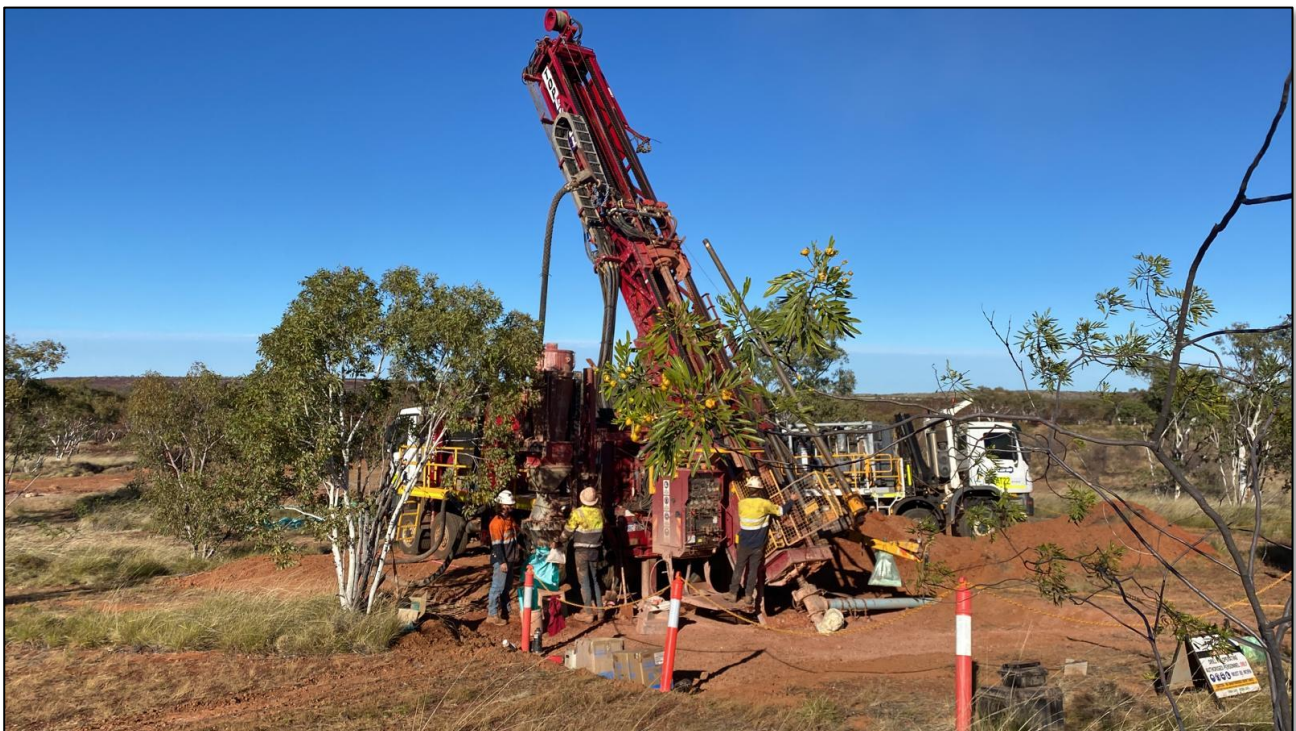
Image 1: Topdrill RC drilling rig testing at Bluebird (BBRC0029)
