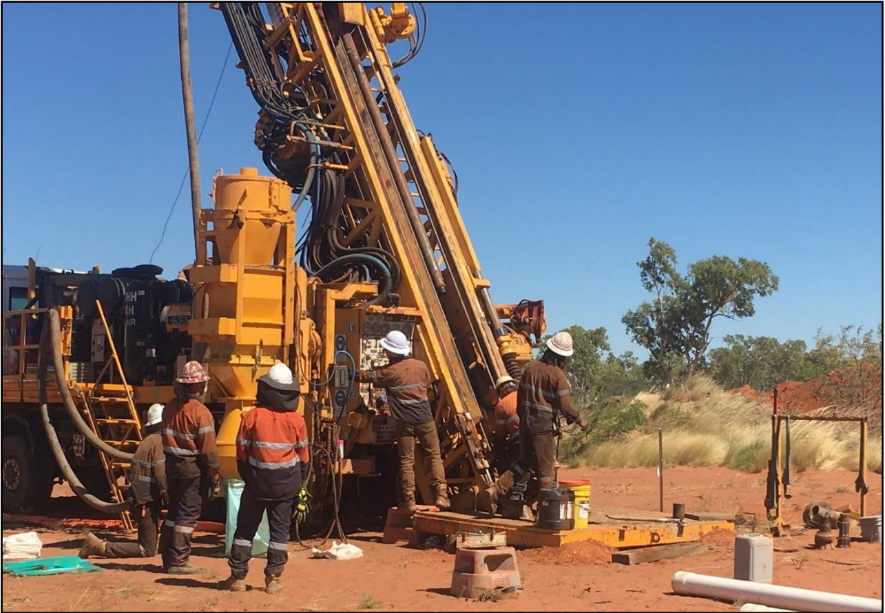
Image 1: DDH1 multi-purpose drilling rig on Stage 3 RC/diamond hole BBDD0026 2
