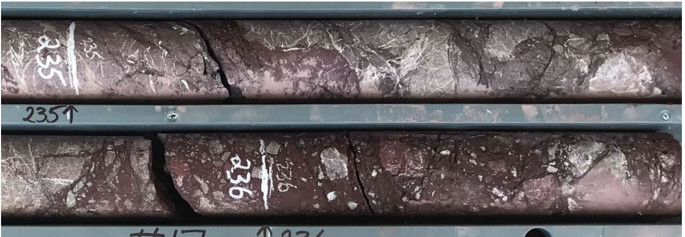
Image 2: Mineralised haematite-breccia in fault zone at Perseverance North, PNDD002, 235 - 236m downhole
