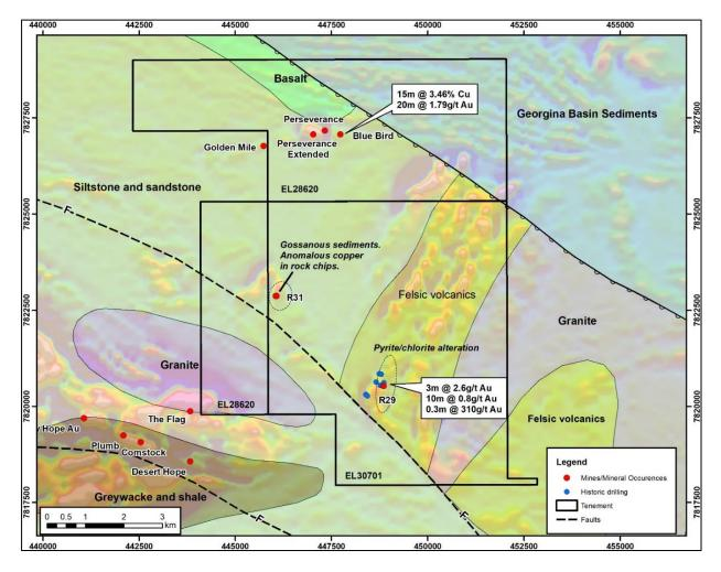
Figure 4: Babbler Project showing regional geology on a TMI aeromagnetic image. Prospects are shown in red.
