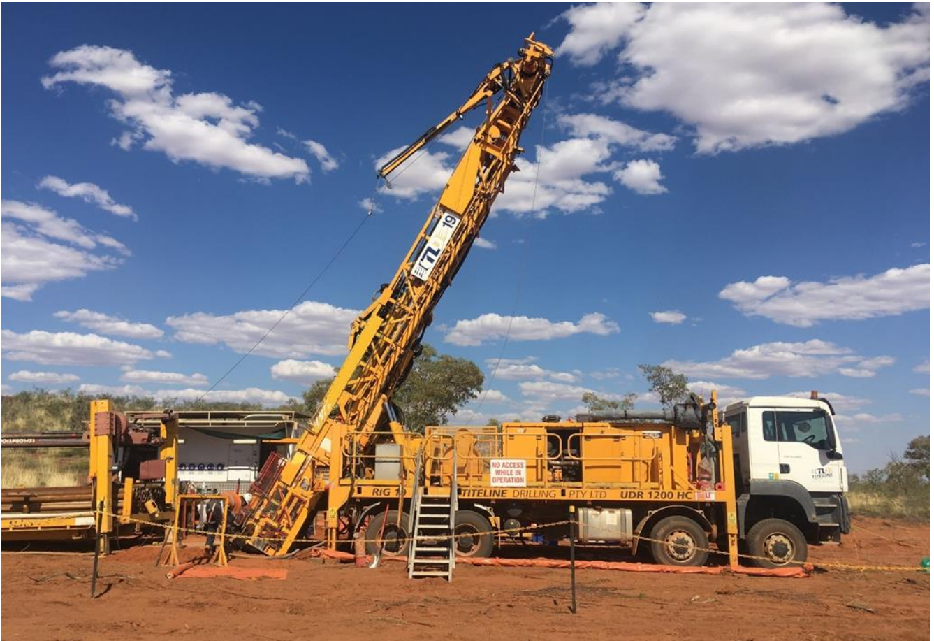
Photo 1: Diamond drilling rig on the BBDD0012 o site at the Bluebird copper-gold discovery
